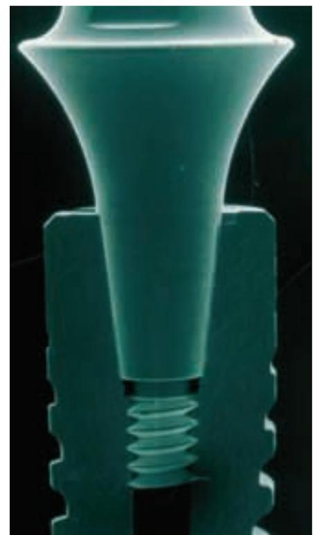
A conically tapered implant abutment connection.
