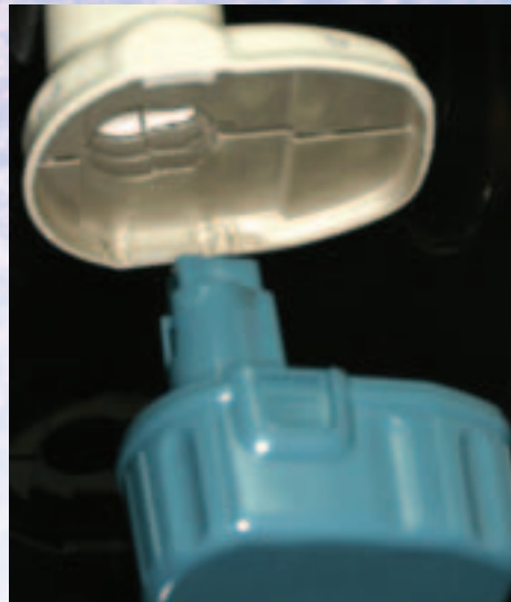
Figure 2-Replacable NiCd batteries insert into the handle
